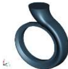
Fig.2: Complete and segment 3D CFD fluid domain of centrifugal pump impeller model.
