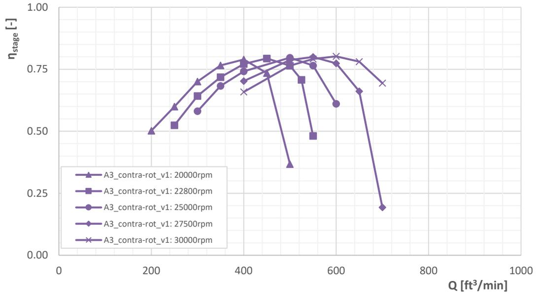
**Figure J: Contra-rotating Axial Fan, Total-to-total Efficiency Comparison (Impeller1, Impeller2)**
