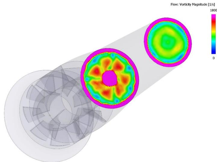
**Figure N: Vorticity Magnitude of Contra-Rotating Axial Fan at 22,800RPM/500 CFM**
