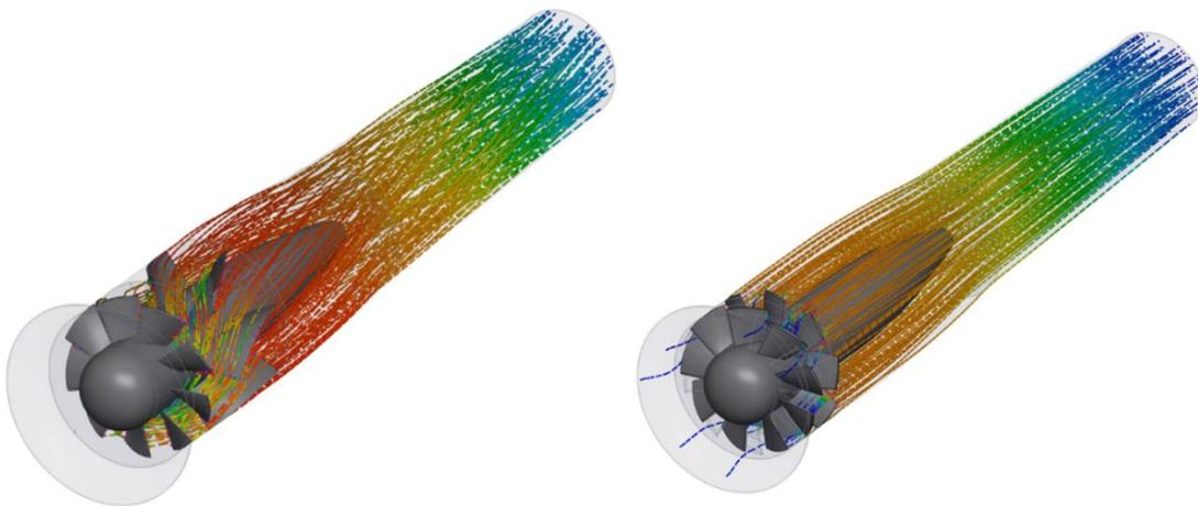
Figure L: Swirl Visualization of Single-stage Axial Fan (Left) at 25,000 RPM/500 CFM and Contra-rotating Axial Fan (Right) at 22,800 RPM/500 CFM
