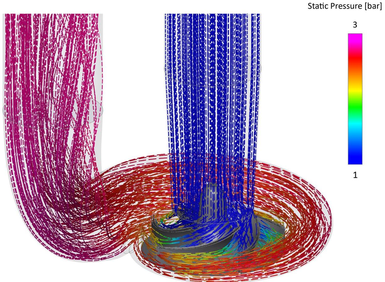
**Figure K:** Static Pressure Streamlines – Optimized4 Design
