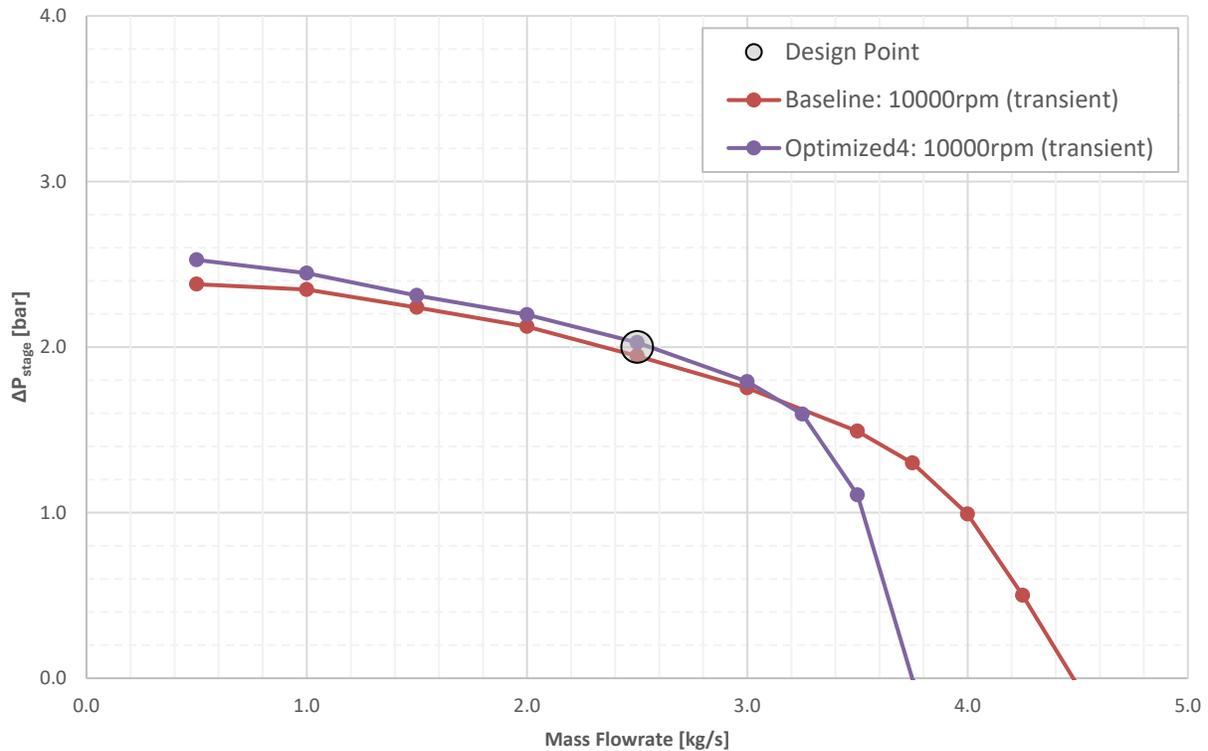
**Figure F: Total Pressure Difference Across Stage – Optimized4 vs. Baseline**
