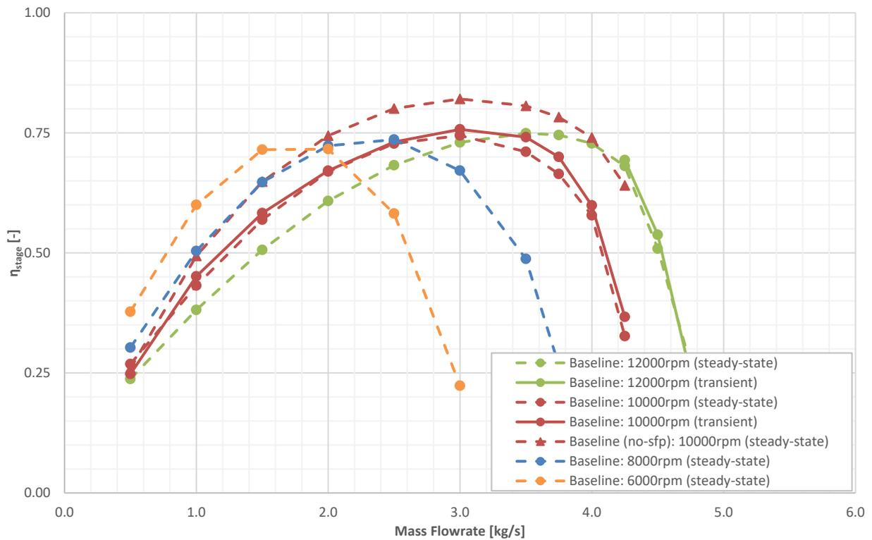
Figure D: Stage Efficiency – Baseline Design
