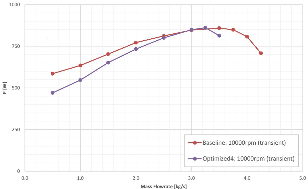
**Figure I: Shaft Power – Optimized4 vs. Baseline**
