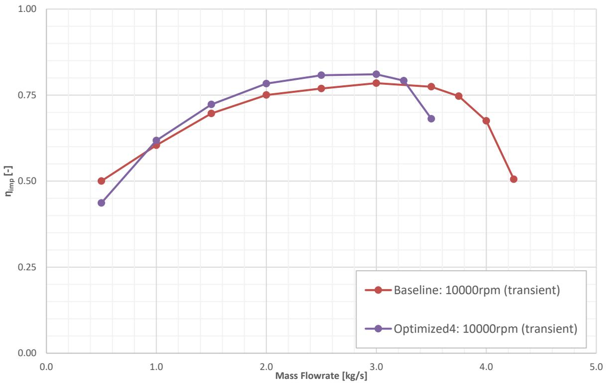
**Figure H: Impeller Efficiency – Optimized4 vs. Baseline**
