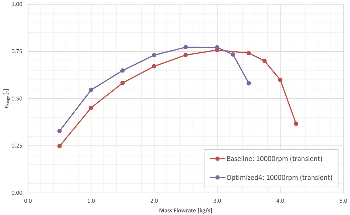
**Figure G: Stage Efficiency – Optimized4 vs. Baseline**
