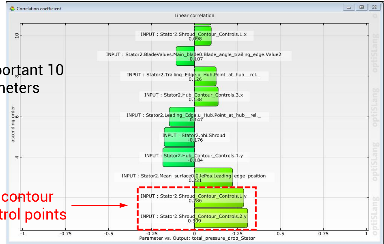
b) Total pressure losses bowl diffuser
